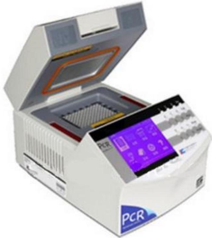
**IN ESSI LE PROVETTE CONTENENTI LA MISCELA DI REAZIONE SONO POSTE IN BLOCCHI DI METALLO RISCALDABILI E LE VARIE FASI DI UN CICLO (TEMPERATURA E DURATA) COSI' COME IL NUMERO DI RIPETIZIONE DEL CICLO SONO PROGRAMMABILI MEDIANTE UN PICCOLO COMPUTER INCORPORATO**
